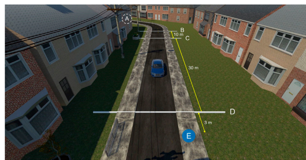
FIGURE 2 The simulation environment used for the HIKER experiment. Each salient point is demarcated by a label, together with the distance (in metres) between each point. (A) spawn point, (B) AR interface onset, (C) AV deceleration onset, (D) stopping point, (E) participant location. Image adapted from Tabone et al. (2023).
