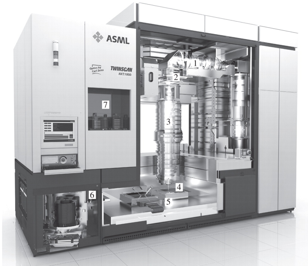
Figure 1.3: Wafer scanner from ASML with the main modules for exposing a wafer. The illuminator (1) directs the exposure light to the reticle on the reticle stage (2). The pattern of the reticle, defined in a chromium layer on a quartz plate, is imaged by the projection lens (3) onto the wafer (4) located on the wafer stage (5). The wafer handler (6) exchanges the wafer after each exposure while the reticle handler (7) exchanges the reticle for each different layer that is required for a functioning IC. ( Courtesy of ASML. )
