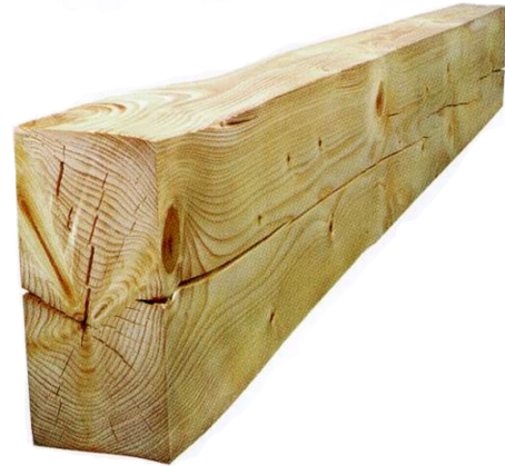
Figure 2.6: Sawn timber beam with pith, knots and drying cracks
