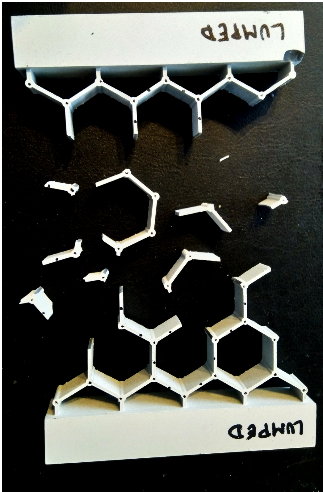
Fig. 9.10 Photograph of the lumped-node honeycomb post-experiment fragments
