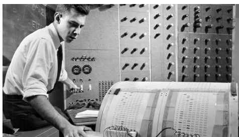
Figure 2.2: Rosenblatt working on the perceptron, the first concept of a neural network, introduced in 1958 [37].
