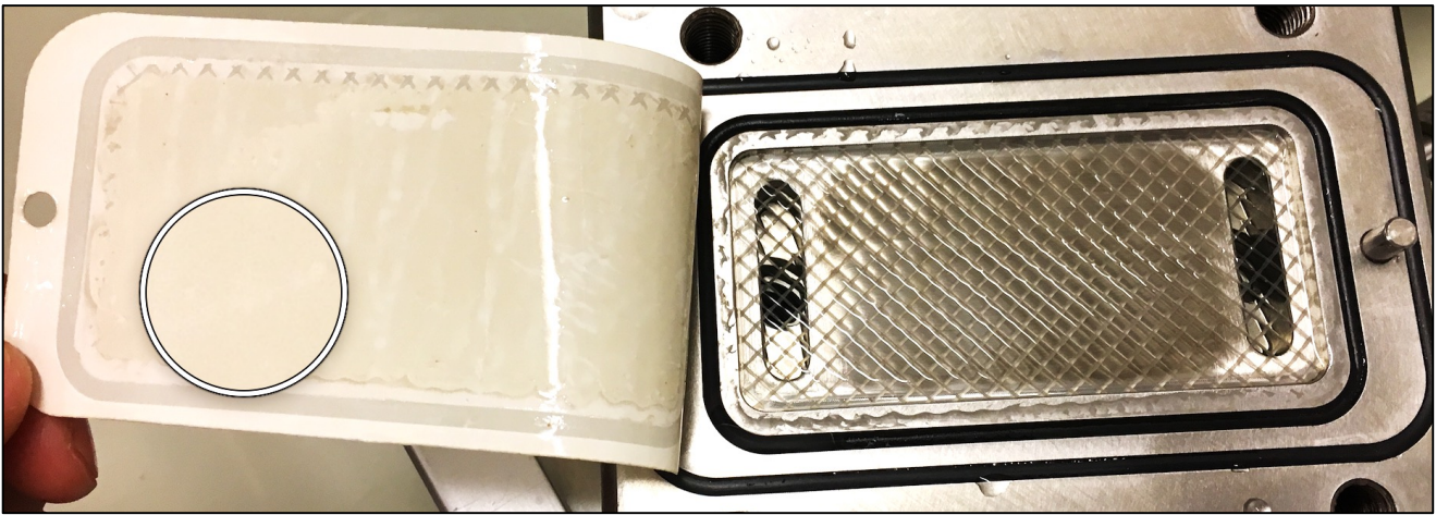
Figure 23: On the right side of the image, crossflow cell with a zigzag spacer and no plastic shim. On the left side, a fouled flat-sheet membrane. The circle on the membrane is a zoomed-in area, showing a homogeneous fouling, proving that the spacer did not comply with its functions.
