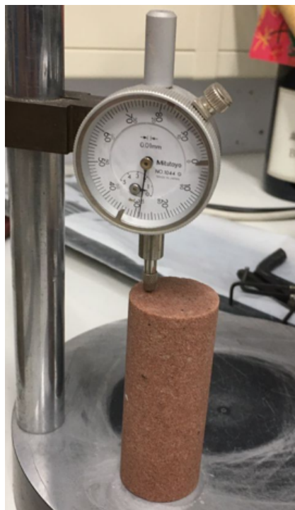
Figure 4.1: Red Felser sample and tilting indicator equipment used to discard samples with ending surfaces that could lead to stress concentration areas during cyclic triaxial tests.
