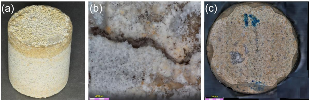
**Fig. 7** **a** Salt crust in Massangis specimens contaminated with 5 wt%  $\text{Na}_2\text{SO}_4$ ; **b** detail of salt crust on Massangis specimen contaminated with 1 wt%  $\text{Na}_2\text{SO}_4$  after brushing off the
