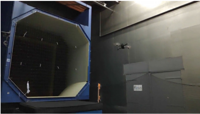
Fig. 12. Snapshot of the tested quadrotor in the wind tunnel, with removal of rotor 1 and 3.
