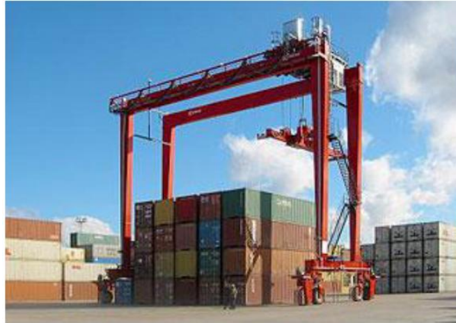
Figure xiii – Rubber tyred gantry (RTG) crane (Quist & Wijdeven, 2014)
