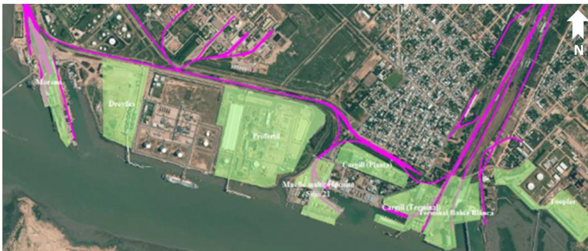
Figure iii - Rail network in the Port of Bahía Blanca, terminals in green are accessible by rail (Arecco, Besson, van Drunen, & Sendra, 2017)
