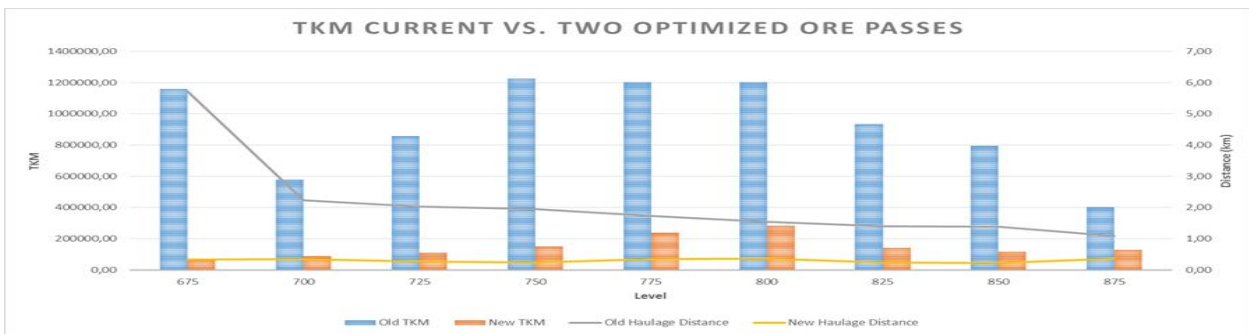
Figure 62 Scenario 2, summary of haulage distances per level compared to the current situation
