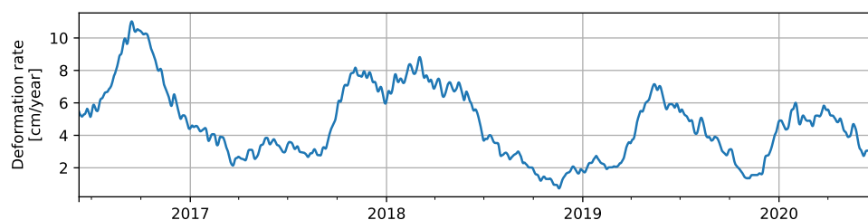
Figure 1.3: Landslide deformation rate at one of the benchmarks, as observed by the automated total station.
