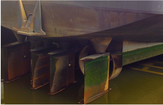
Figure 1.1: An inland vessel with a hull tunnel, ducted twin propellers, and quadruple rudders.
