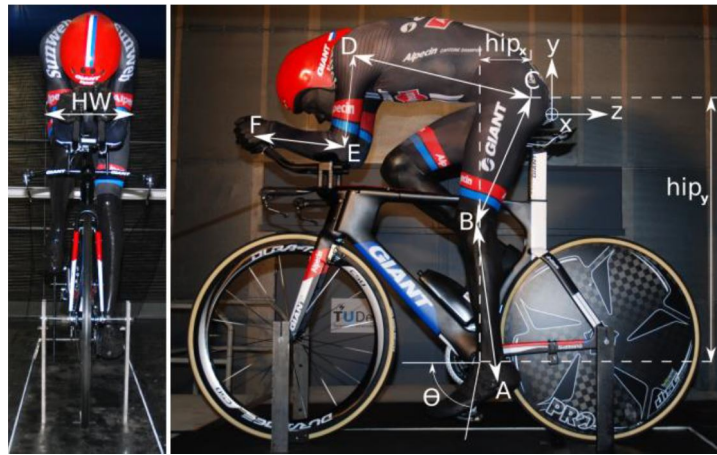
Figure 3.2: Dimensions of the mannequin (Reproduced from Terra et. al. [67])
