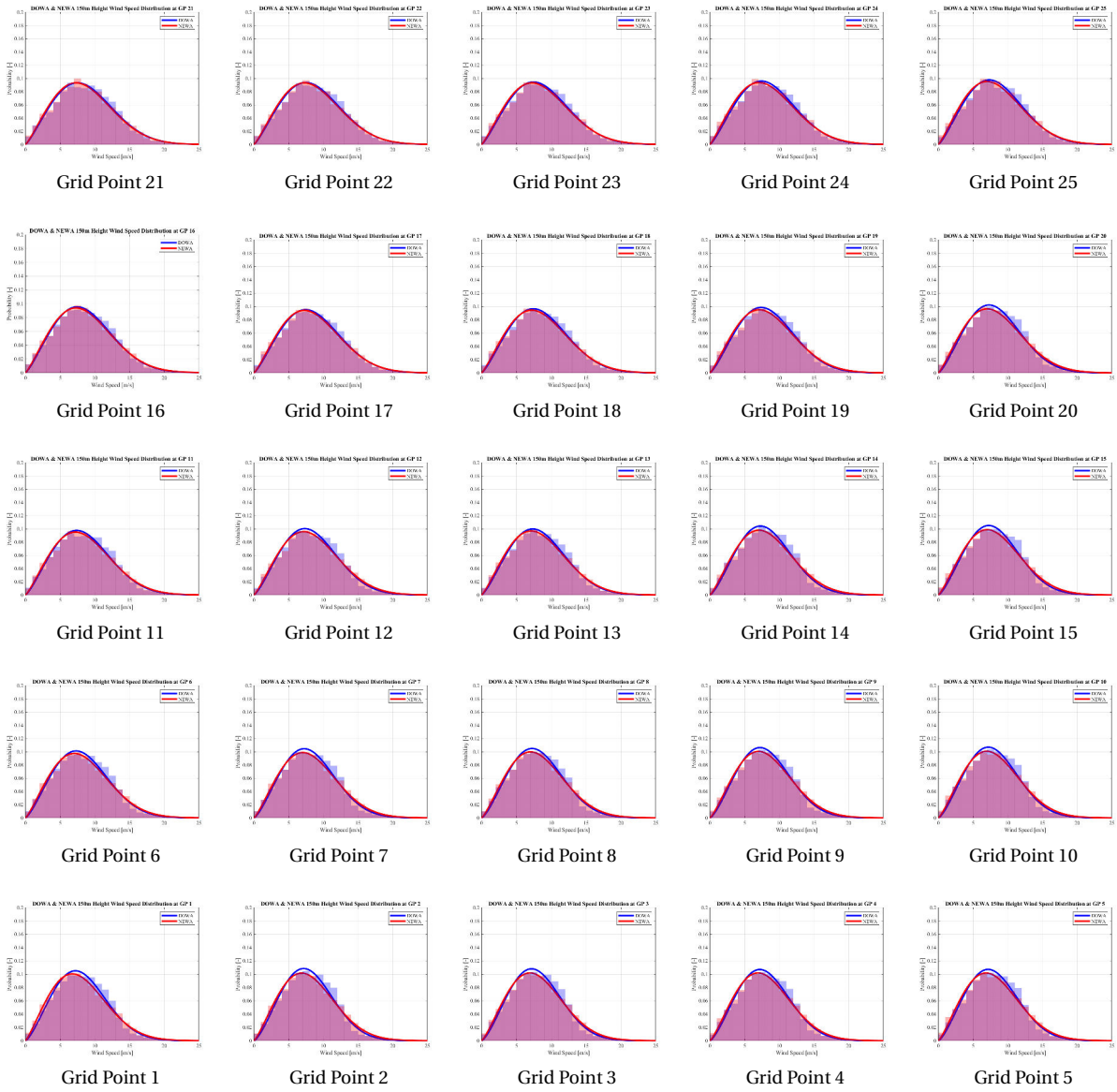
Figure A.3: PDF plots of DOWA & NEWA data for 25 grid points at 150m height.
