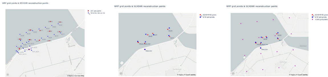
Figure 5.1: Left: Original site layout of WRF grid points and SCADAR reconstruction points. Center: Site layout after filtered out considerable distances. Right: Site layout after NEWA grid points are added.
