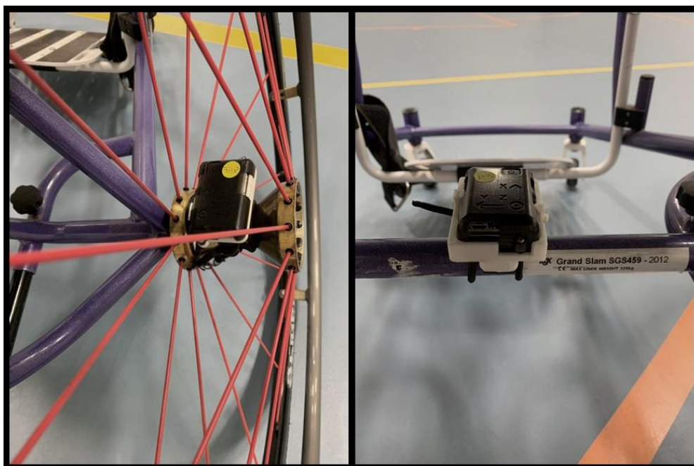
Figure 2: Placement of sensor right wheel (left picture) and on frame (right picture)
