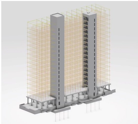
(A) Concrete cores [36]
