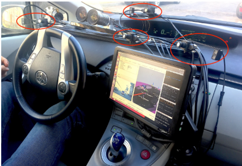
Figure 4.1: Interior of the vehicle showing the four eye-tracker cameras encircled in red, and the built-in display used for the post-drive recognition task.
