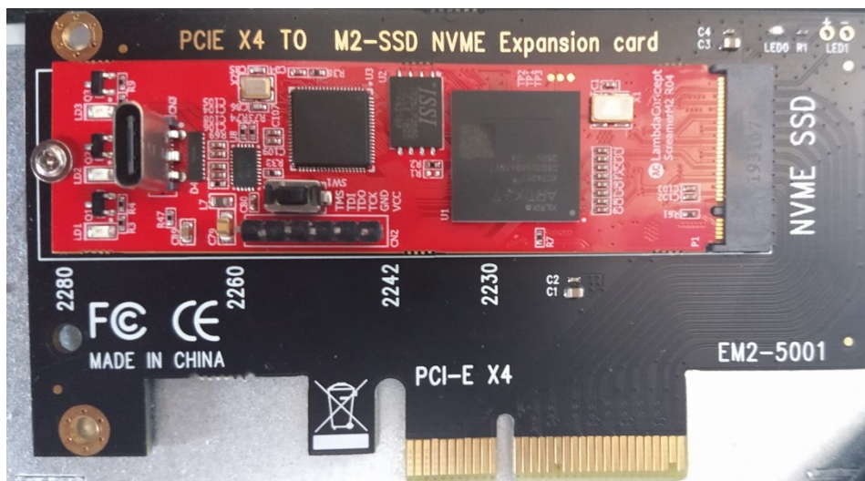
Figure 6.1: The PCILeech M.2 Card in a PCIe x4 Adapter
