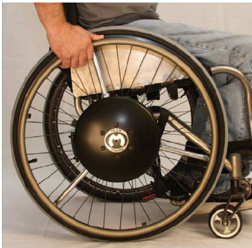
Figure 4: An Instrumented wheel from Optipush (Guo et al., 2011)
