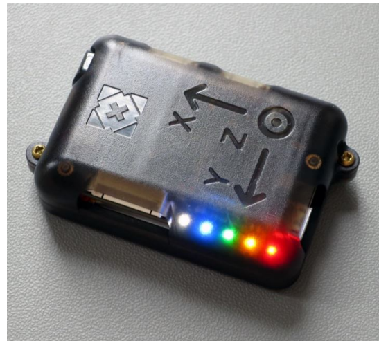
Figure 5: New Generation Inertial Measurement Unit (X-ioTechnologies, 2021)
