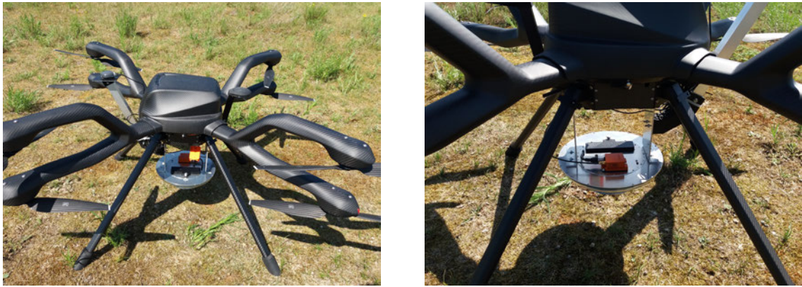
Figure C.4: The image on the left shows a photograph of the drone and radar system with the GNSS antennas visible. The radar mounted camera is also visible. The image on the right shows the radar system mounted to the drone. In the image, the Xsens G710 INS is also visible as the red module on top of the radar.
