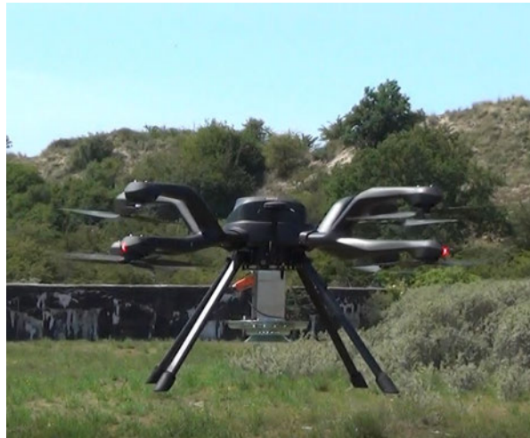
Figure C.2: The radar system mounted to a multi-copter platform hovering above the ground.
