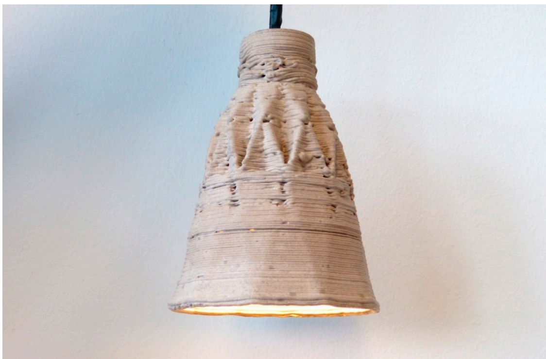
Figure 1. Lampshade 3D printed with a composite material from mussel shells and sugar water (design from Joost Vette).
