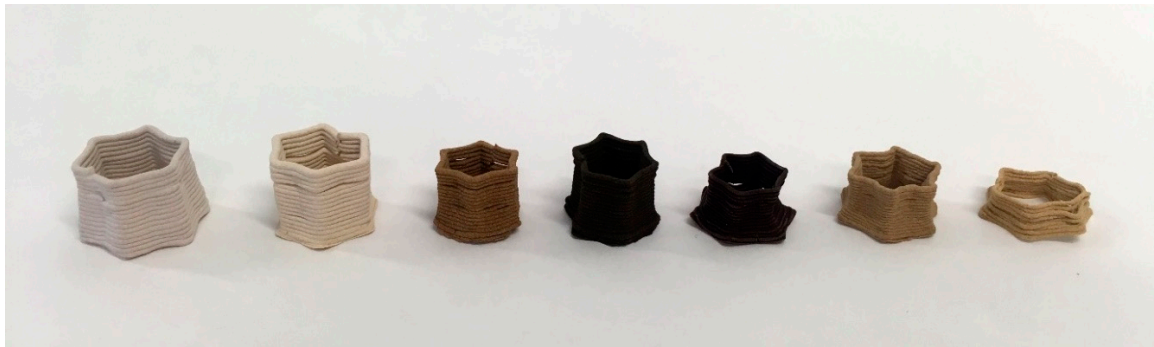
Figure 6. 3D prints with a variety of fillers, from left to right: mussel shell, eggshell, walnut shell, olive pomace, cacao shell, maple sawdust, and pine sawdust.
