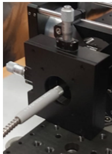
Figure 3.18: Photo of a fiber alignment stage, which is used to mimic relative movement between the plasma image and the fiber aperture, at the fiber aperture, to measurement when the plasma image is not fully observed anymore.
