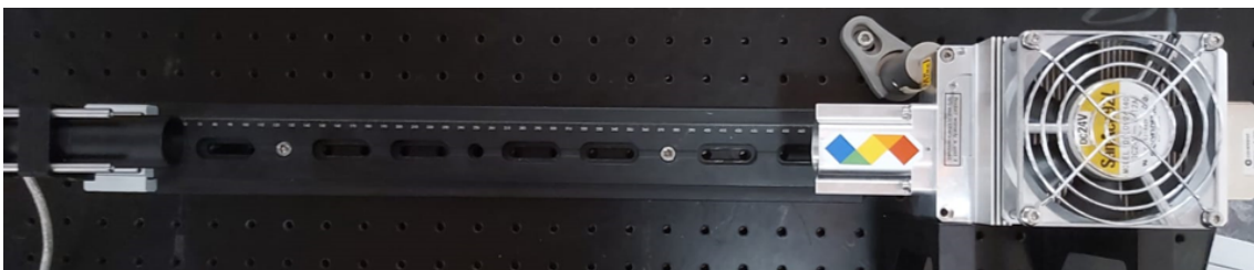
Figure 5.9: Top view photo of the set up to align the beam expander with the laser head.
