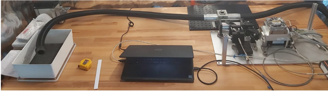
Figure 3.15: Photo of the test set up representing the material flow on the drill rig. Sample input showed to be too random to be able to create a constant plasma and condense the stability requirements.
