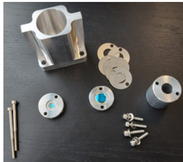
Figure 5.2: Photo of all parts needed for the assembly of the beam expander.
