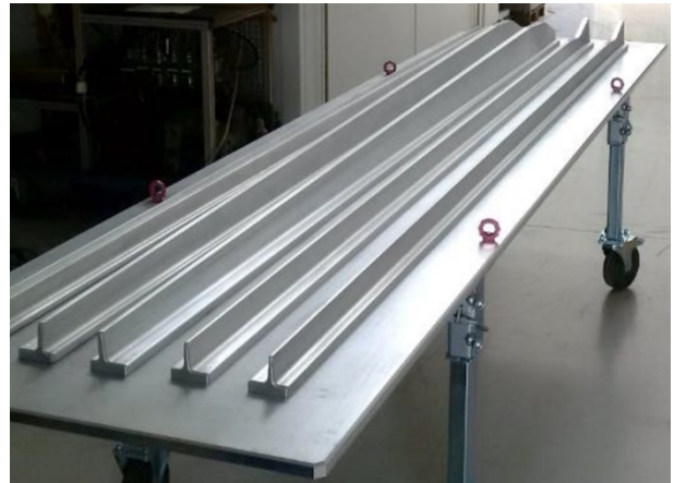
b.) Metal moulds for the front and rear spars
