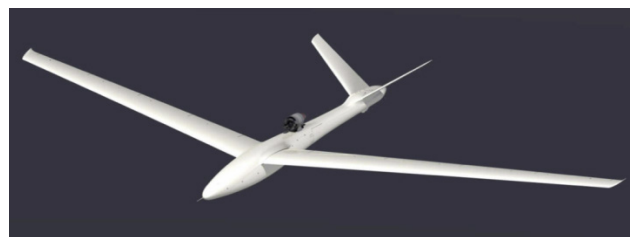
Figure 1: Schematic of the FLEXOP UAV demonstrator
