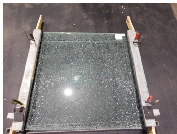
Fig. 9: Disintegrated fully tempered glass top-layer
