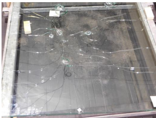
Fig. 6: Cone cracks with cracks extending from them in the heat-strengthened glass after multiple impacts
