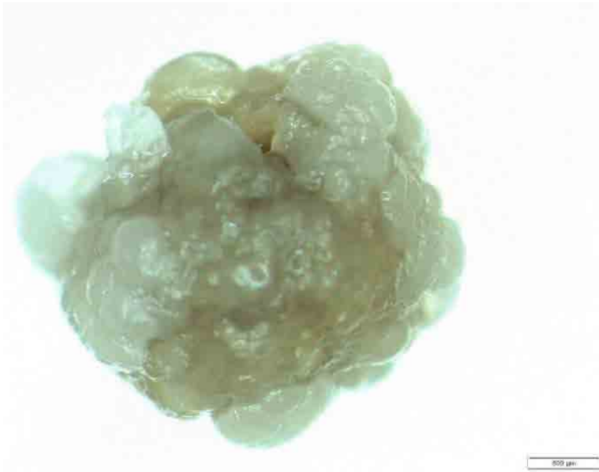
Figure 1.2. Aerobic granule cultured in a laboratory-scale reactor captured by optical microscopy, bar 500 \mu\text{m} .
