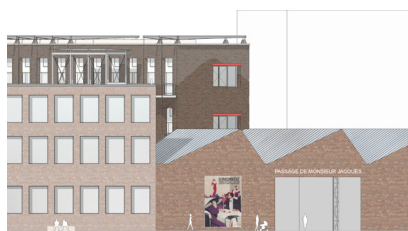
Southwestern Elevation 1:1000 The entrance to the passage occurs through a covered public space.
