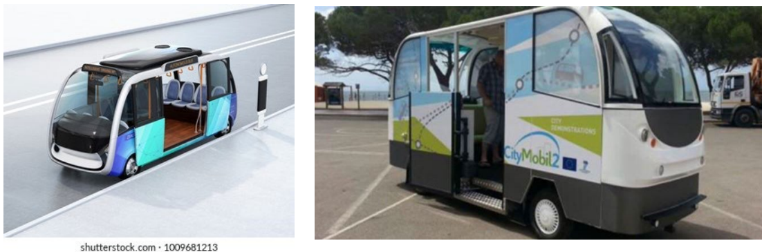
Figure 3 – Example of interior of highly automated “driverless” shuttle with no driver controls (left) and the Citymobil2 shuttle (right, Merat et al., 2016)
