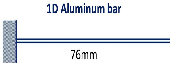
Figure 3.10: 1D beam model used in the analyses shown in chapter 3.4. Temperature variation in the thickness direction and the width direction are ignored and only the variation in the length direction is considered in this 1D model.
