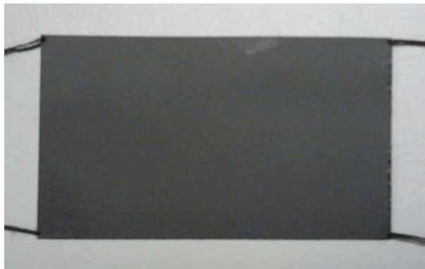
Figure 8.4: Aluminum substrate used in the experimental setup. The aluminum substrate is painted by black paint on both sides to increase heat absorption of the projector light and to reduce the reflection of the radiation from the IR camera which is then measured as measurement error by the IR camera. At each corner, small hole is made and a string hangs the substrate through the hole.
