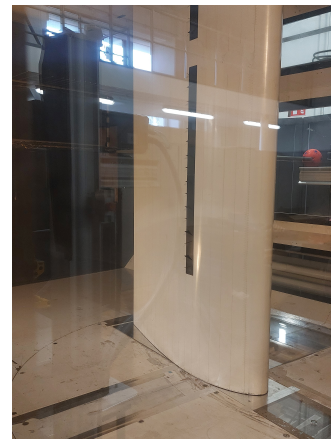
Figure 2: Airfoil model with VG strips
