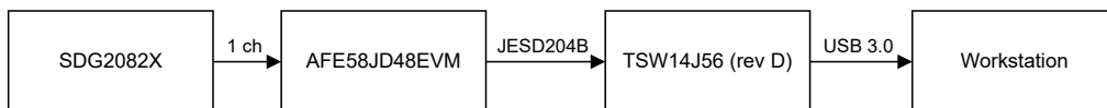
Figure 5.12: Block diagram of the measurement setup used for the testing of the decimation filter parameters.
