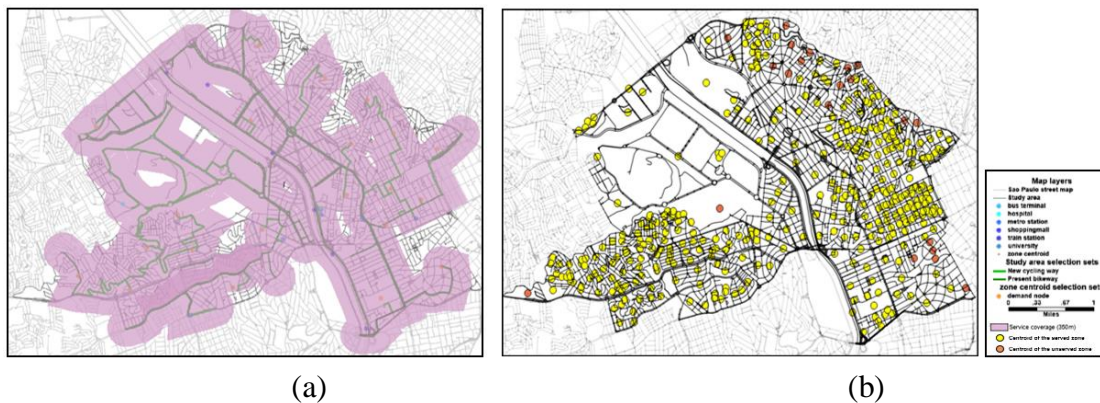
Figure 7. Service coverage of the new cycling network (a) service zone; (b) centroids of the served and unserved zones
