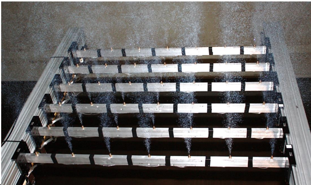
Figure 2. NLR's HFSB 42-bubble generators seeding rake.
