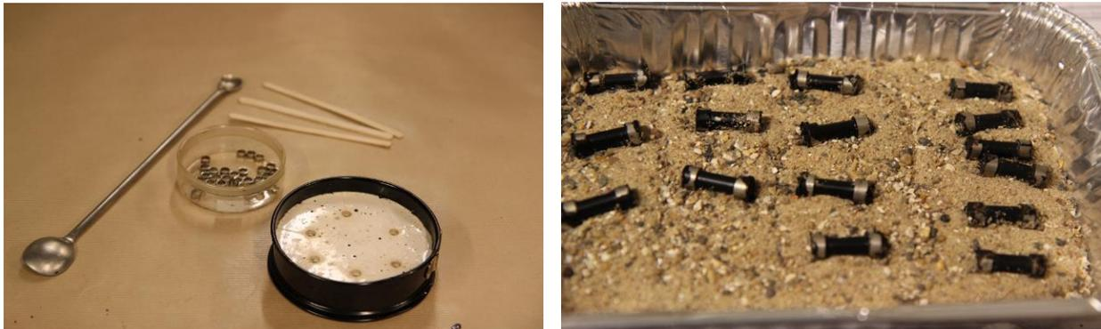
**Figure 3. 4:** Silicon mould and metal rings (left) and storage of the specimens (right)
