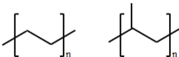
**Figure 2. 2:** Structure of polyethylene and polypropylene [17]
