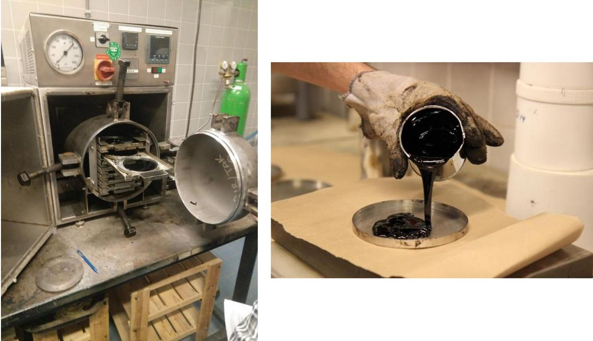
**Figure 6. 2:** PAV aging apparatus (left) and metallic tray (right)
