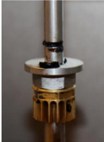
**Figure 5. 2:** Fatigue test and crack initiation of the specimen
