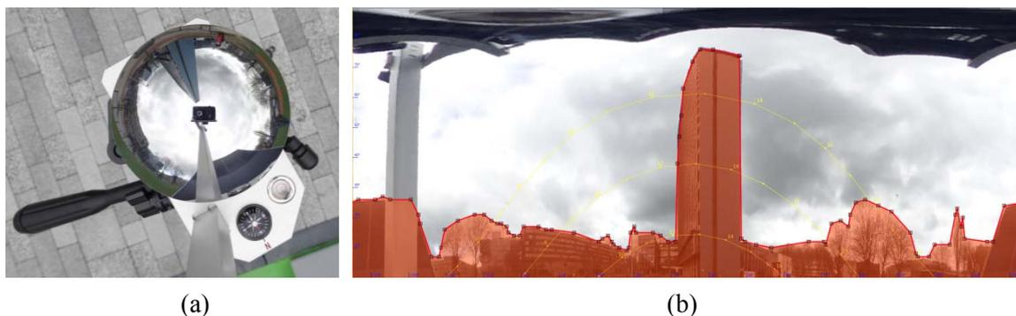
Fig. 4: (a) The Meteororm Horicatcher is used to estimate the (b) shading due to nearby buildings at the location of the e-bike charging station
