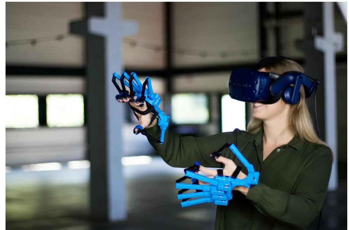
image / figure 2: Senselglove interaction technology with haptic feedback integrated with VR Headset
