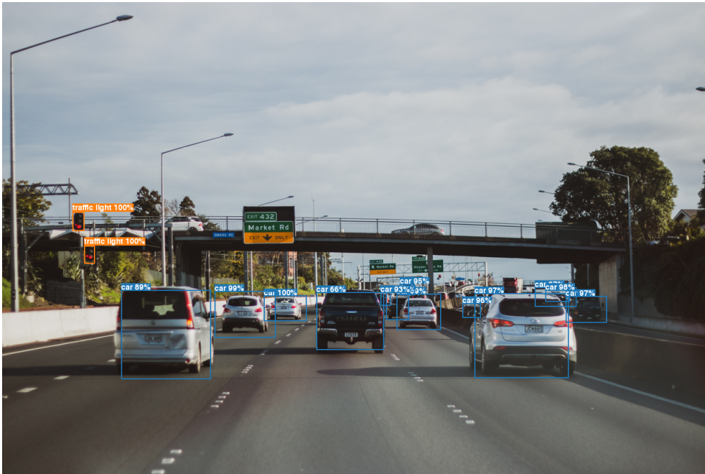
Figure 2.4.: Example of object detection using pre-trained YOLOv3 detection model. Image taken from Ethan Hooson, Unsplash, and processed with the detection model.
