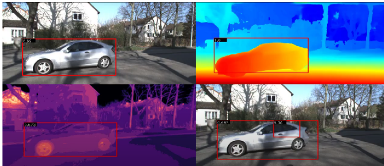
Figure B.1.: Example of inference from 3 teacher networks (RGB on top left, depth on top right, thermal on bottom left) and an audio student network (bottom right).
