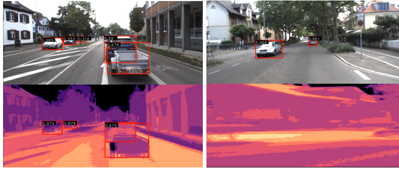
Figure B.4.: An example of 2 RGB images (top) in the dataset and respective correct (bottom left) and corrupted (bottom right) thermal images.
