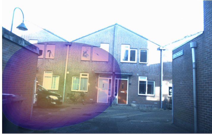
Figure 2.2.: Visualization of a beam over an incoming car. The beam is overlaid on an image captured by the front camera mounted on an ego vehicle.
