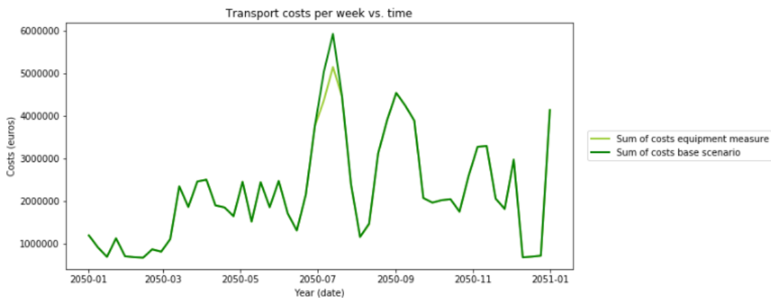
Figure 5.11: Differences in weekly costs with and without equipment measure in the RUST-scenario
