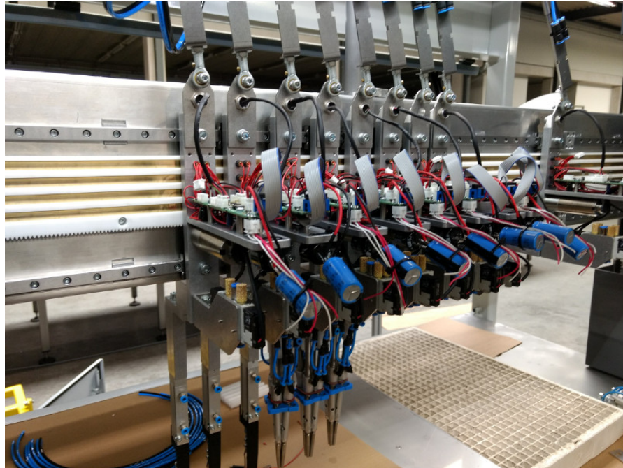
Figure 4.8: Set of mounted grippers without casing
