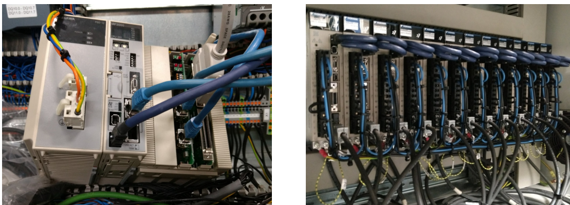
Figure 3.1: Servo drive hardware used in the old Transplanter
