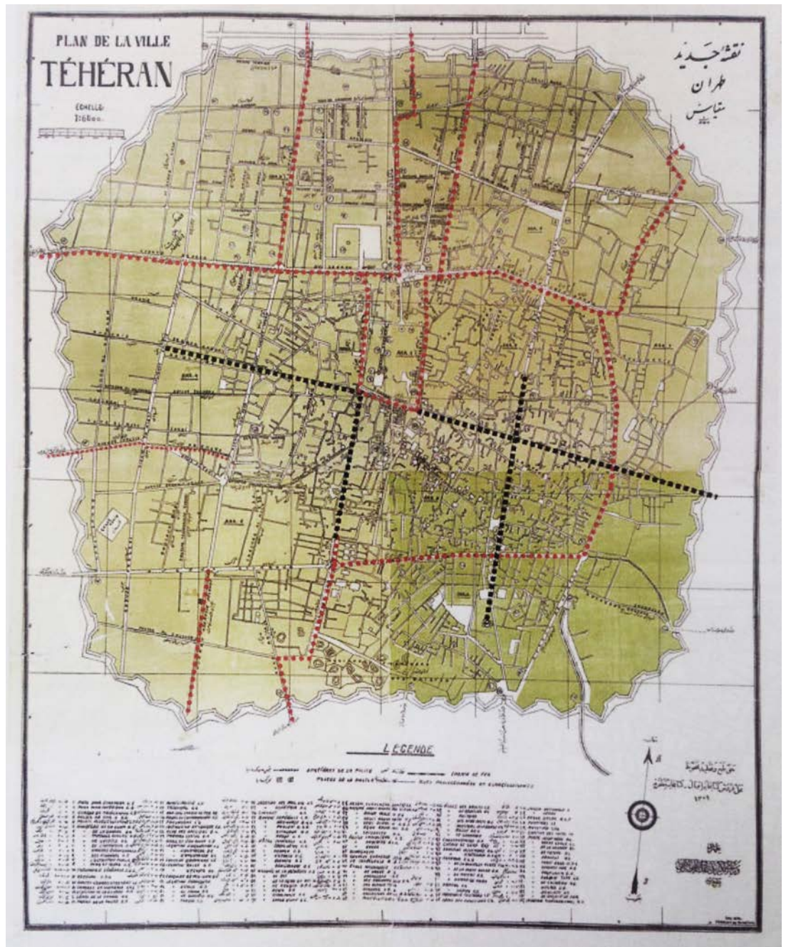
Figure 3.9. Tehran Street Layout Plan 1930 - The Black dotted line shows the new streets and the red dotted lines show widening of the existing streets
