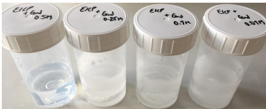
Figure 25 - Test tube EICP reactions diluted with varying Guanidine Hydrochloride concentrations, mimicking residual guanidine ions between the two treatment phases. Murky solutions and wall calcification show EICP occurring at \leq 0.25\text{M} tests.
