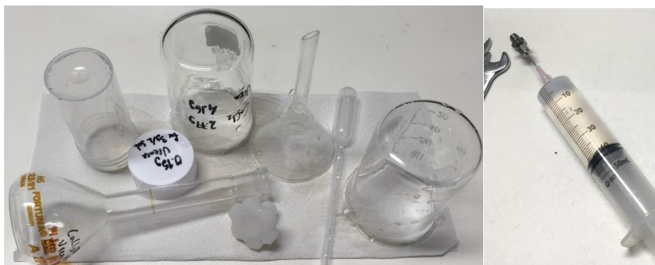
Figure 70 - Time minimization via rapid dilution in a 50mL volumetric flask of urea:CaCl 2 reagents (glass beaker) and dissolved urease (white cap). On the right, an immediate transfer of EICP solution to the DB 50mL syringe.
