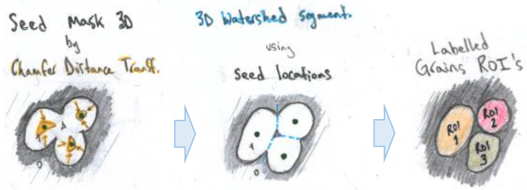
Figure 80 - Step process of individual grain segmentation. Firstly, a chamfer distance transform is applied to the binary (left) to locate the center of each sand/carbonate/void. Secondly, watershed flooding is performed towards the known center points of grains (middle), such that each grains are separated at the catchement split. Thirdly, a label image is generated containing all the regions of interest (right), ready to be analyzed.
