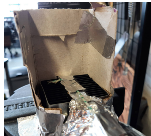
Figure 66. Cardboard windshield placed on top to improve temperature measurement of outgoing air
