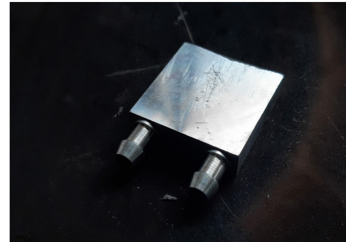
Right figure 59: the aluminium water cooler.
