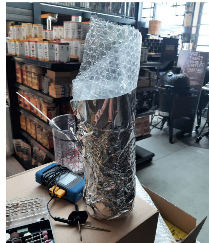
figure 60: the container with water, properly insulated with both bubble plastic and aluminium foil.
