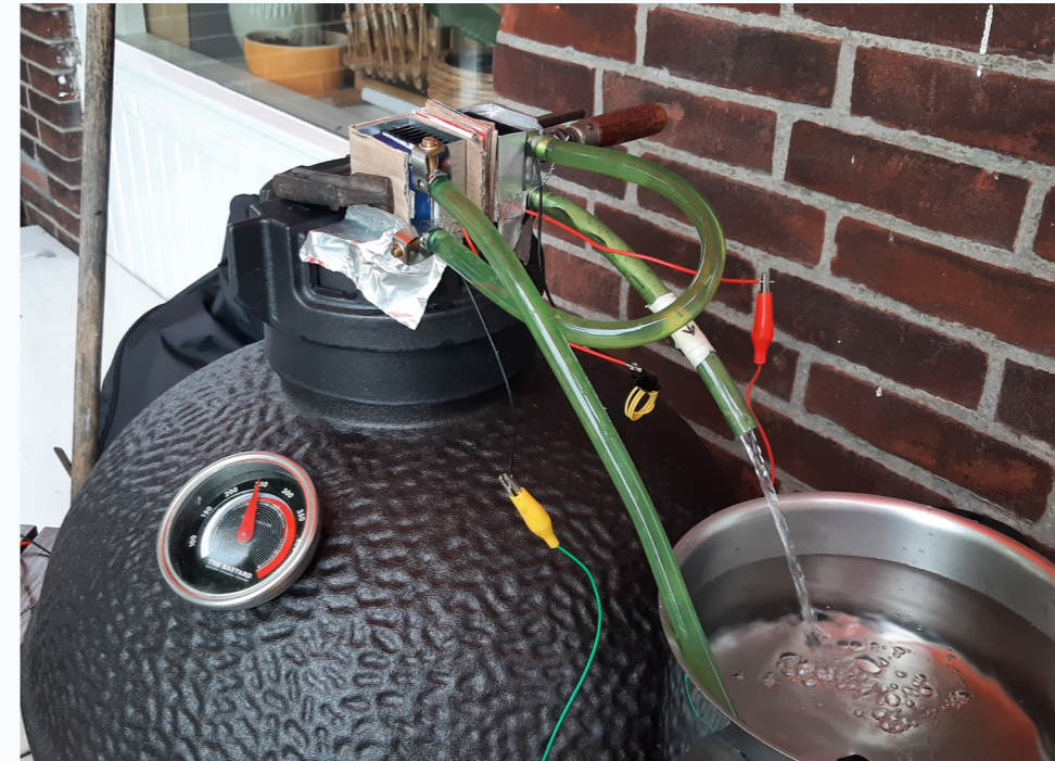
Figure 49. Test setup Peltier element experiment
