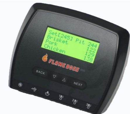
Figure 28. The interface of the FLAME BOSS 500
