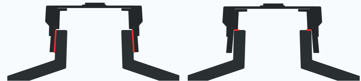
Figure 39. The old closing vs the new closing principle. When flat cast iron surfaces touching each other close off the cap, it is easier to make it airtight.
