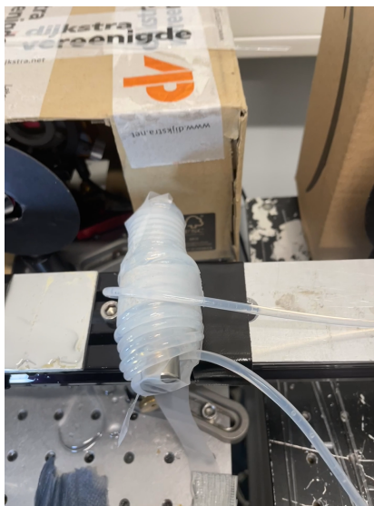
Figure 3.3: FEP tube coil in the microfluidic setup.
