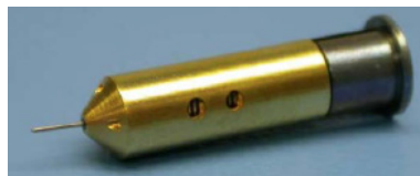
Figure 5.9: Single ST-7 Colloid Thruster Emitter [40]
