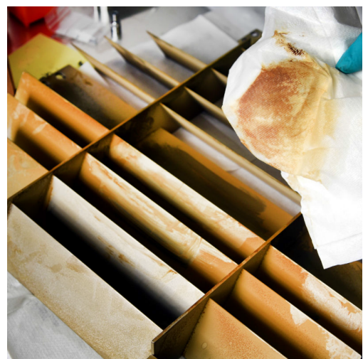
Figure 4.31: First Stage Shield Iodine Reactants Cleaning [4]
