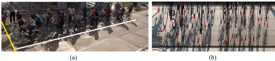
Fig. 4. Example of a queue showing the cross-section (yellow) and queue length (white) that is used for the analyses (a) and the constructed image in space and time (b) showing the lateral position and passing time of all front wheels indicated with red dots. (For interpretation of the references to color in this figure legend, the reader is referred to the web version of this article.)
