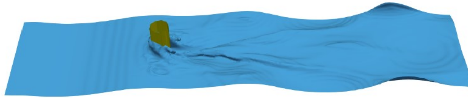
Figure 4.12: Simulated free surface in blue and cylinder in yellow at t = 2 s, with U = 4.02 m/s and regular waves with T = 1.48 s and H = 0.14 m
