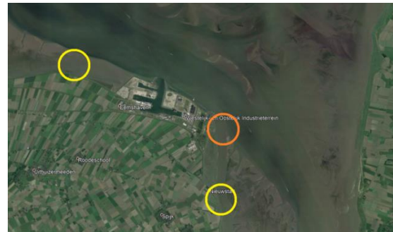
Figure 2 - Potential wave run-up and wave overtopping measurement locations (yellow circles) and potential water level, current and wave measurement locations (yellow and orange circles).
