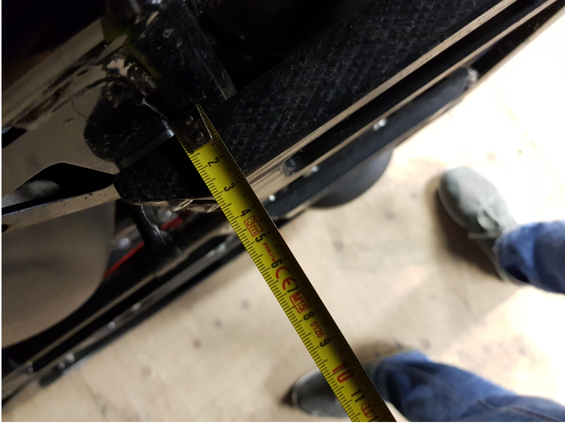
Figure 2.5: Height of rental go-kart and plastic buffers.
