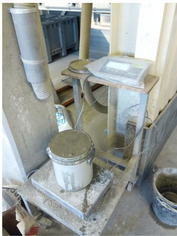
Figure III.7: Measuring of the density
