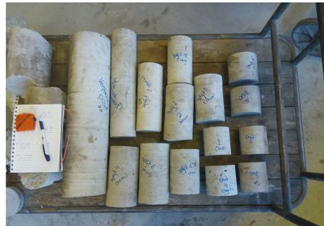
(b) Sawn drilled cores provided
