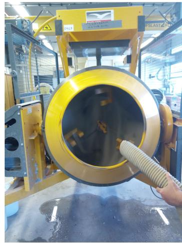
(b) Mixing of the dry sand fractions
