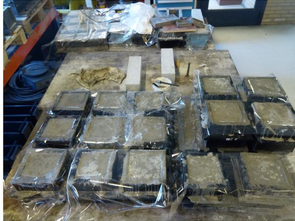
Figure III.9: Several casted specimens
