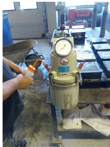
Figure III.8: Measuring of the air content
