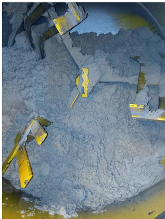
Figure III.2: Mixing step 2: saturating sands (replicating soil)
