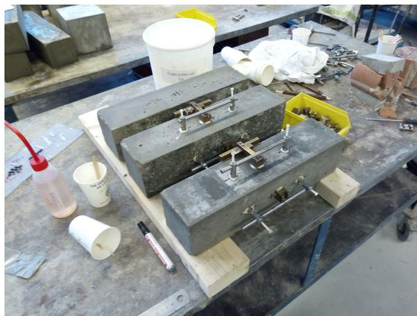
Figure V.7: Attaching the LVDT's
