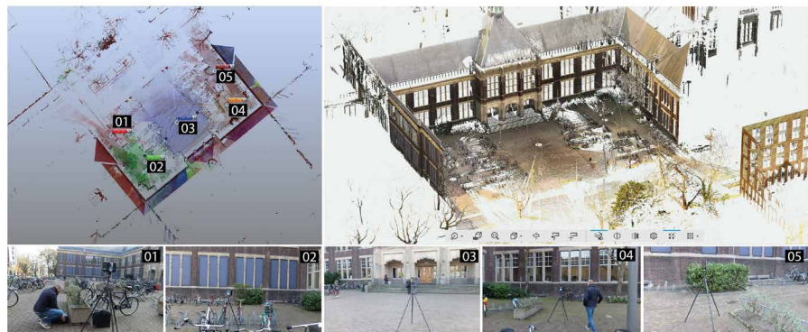
FIG. 5.4 Dataset collection and the different views captured in relation to the scanning position
