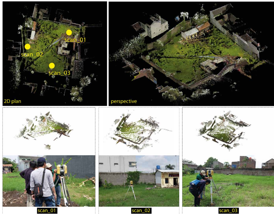
FIG. 5.21 Dataset collection with different views captured in relation to the scanner position
